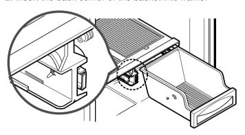
Slightly tilt up the front and push back until it snaps into place.
